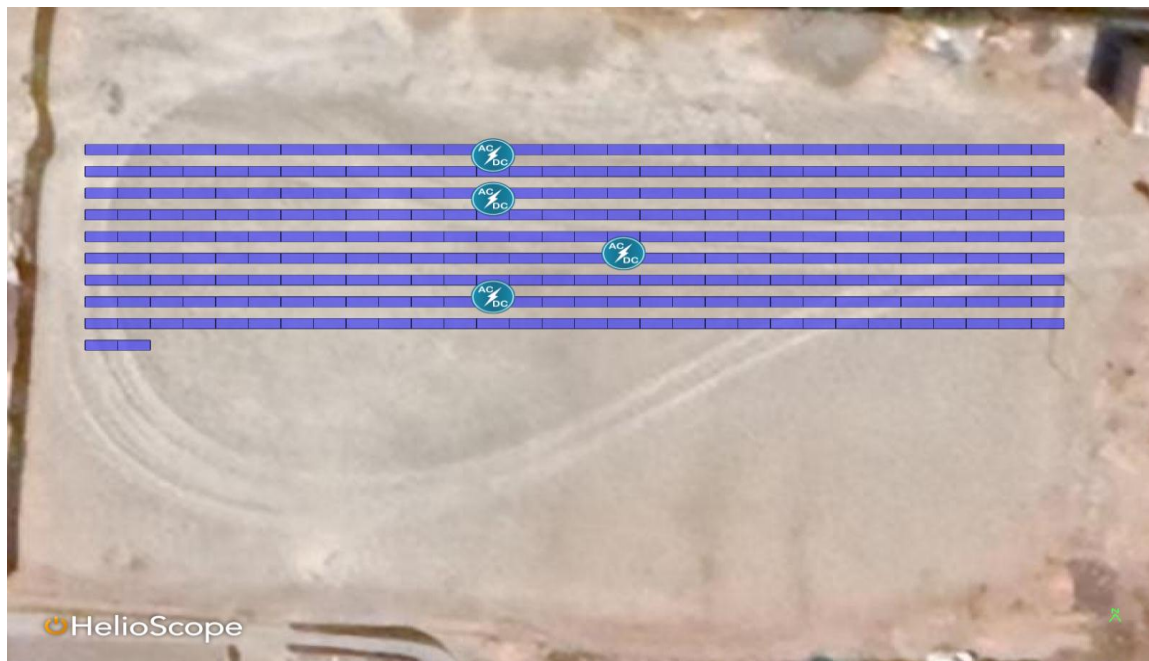
Figure 39: design de l'installation
