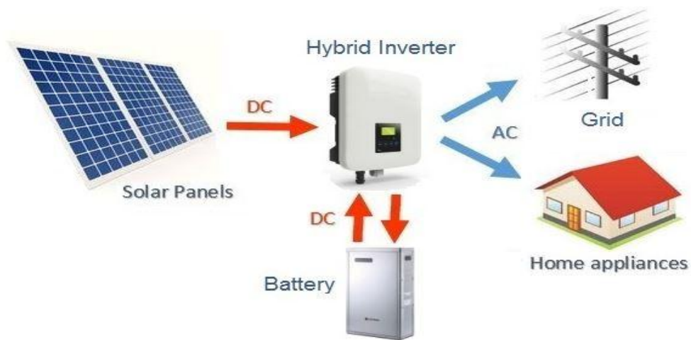
Figure 26: installation photovoltaïque hybride
